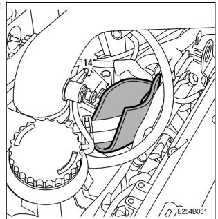
15 Install the crankcase ventilation hose so that the check valve is located above the coolant hoses. The crankcase ventilation hose must follow the route of the lower coolant hose through the intake manifold and then on to the oil trap.
