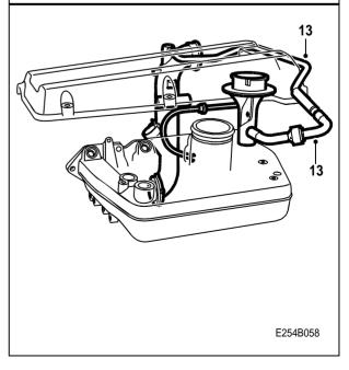
14 Install the insulation under the throttle body coolant hose so that the insulation's short sides point upward.
